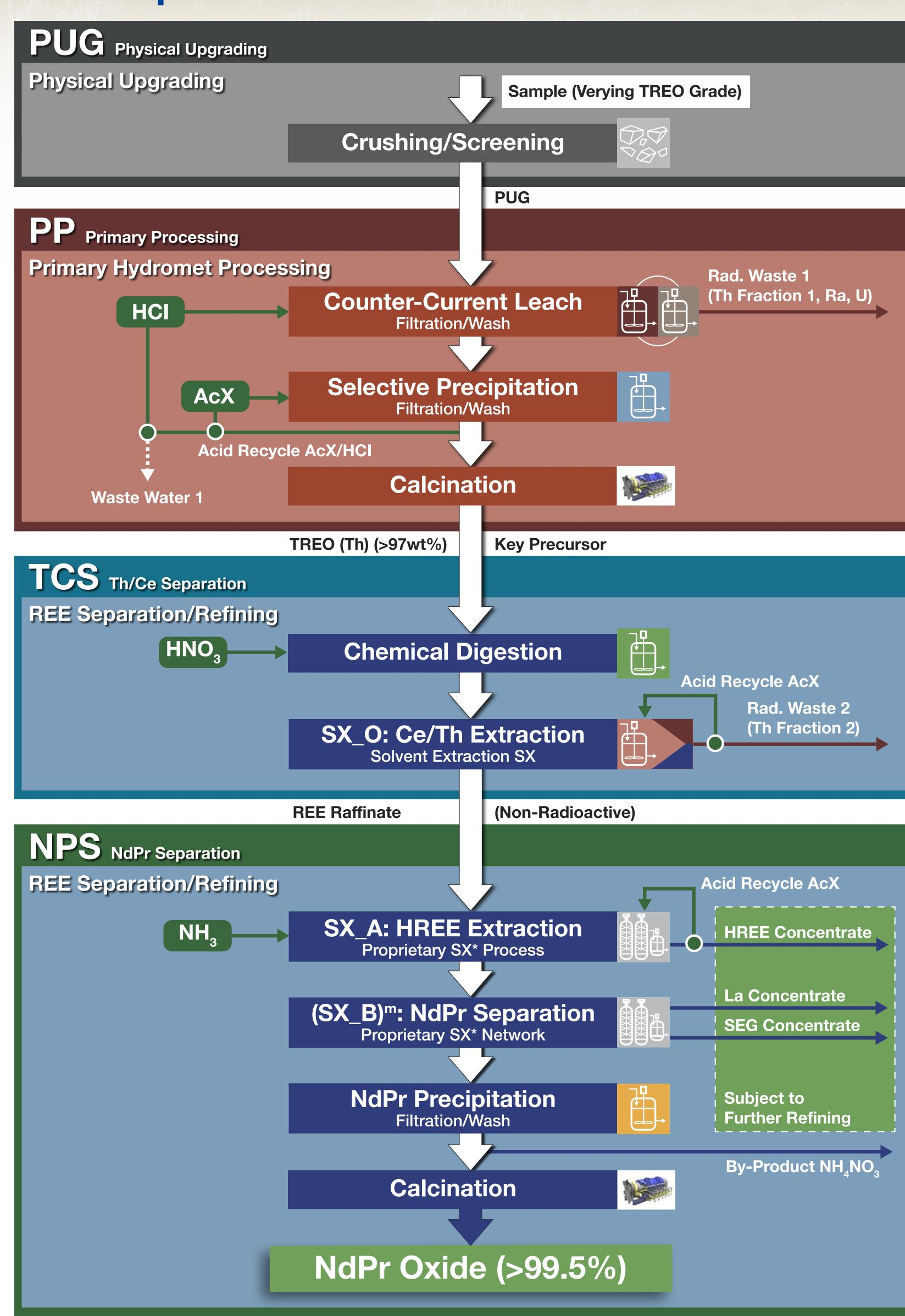
**PUG Physical Upgrading** or comminution of the exploration sample; crushes sample to 1-3 mm size for further processing
