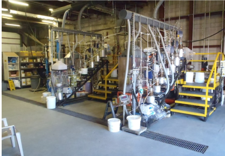
Figure 13.13 - Counter Current Leach ( 30 kg/day) and Precipitation Units
