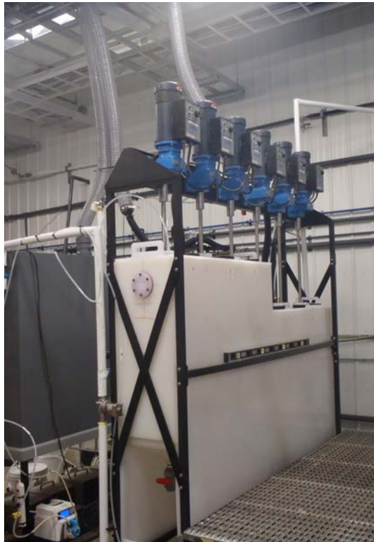
Figure 13.15 - Pilot Precipitation Apparatus at SGS – 2013
